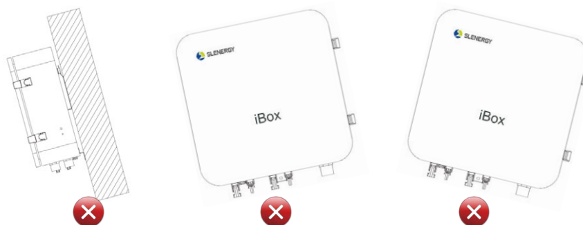
Wrong installation tilts
