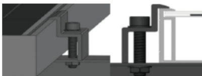
Installation of side fixture(≥50mm)
