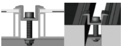
Installation of middle fixture(≥40mm)
