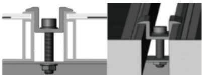
Installation of middle fixture(≥40mm)
